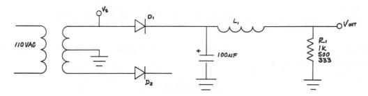
CIRCUIT #6: Full-wave rectifier with PI filter
