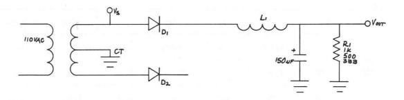
CIRCUIT #5: Full-wave rectifier with inductive input filter
