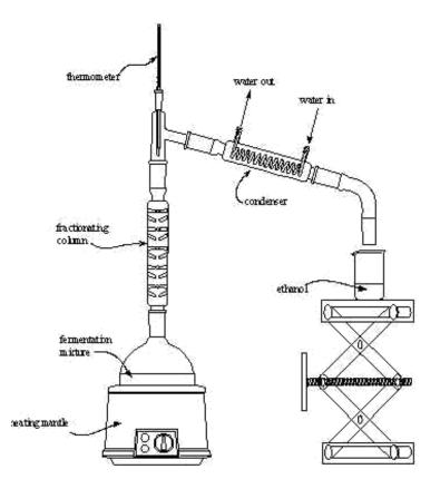
In a process similar to that of crude oil, the ethanol/water mixture can be separated by fractional distillation because of the difference in boiling points.
