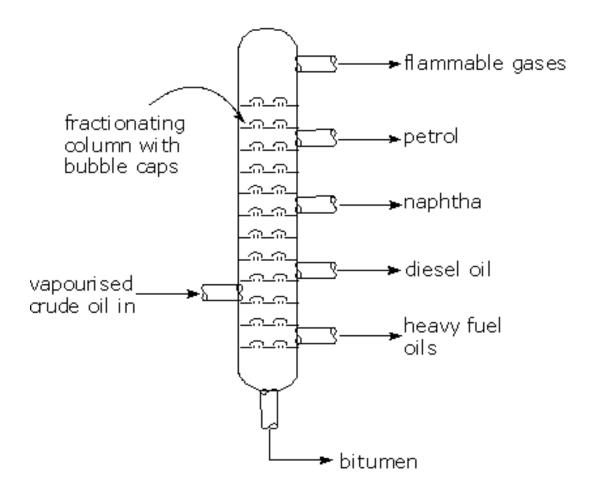
The vapours with the lowest boiling points pass all the way up the column and come off as **gases**, **e.g.** methane, ethane and propane. The temperature of the column gradually decreases the higher up the vapours go, and so various fractions will condense to liquids at different heights. The fractions with the highest boiling points do not vaporize and are collected at the bottom of the fractionating column, e.g. bitumen
