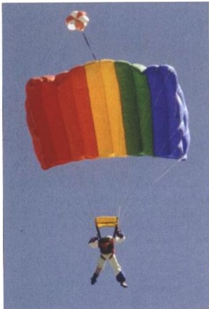
The parachutist descends slowly, with the air resistance on the parachute causing it to pull upwards with a force exactly equalling the parachutist's weight.
