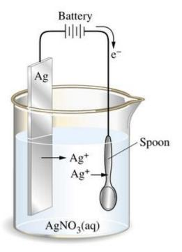
Electrolysis can be used to form a very thin coating of a metal on the surface of another metal object. This can be used for decorative purposes or for protection against corrosion.
