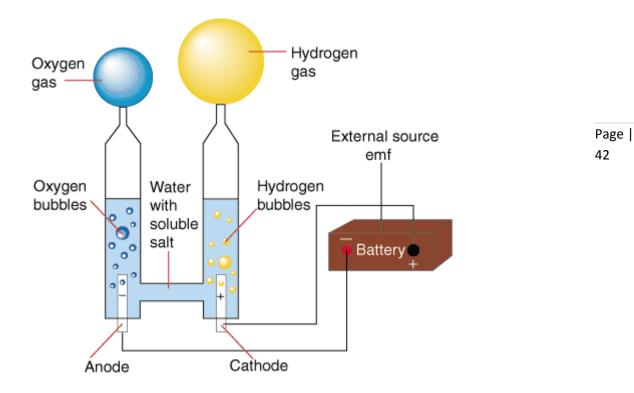
Pure water is a very poor conductor of electricity. However it can be made to decompose if some dilute sulphuric acid is added.
